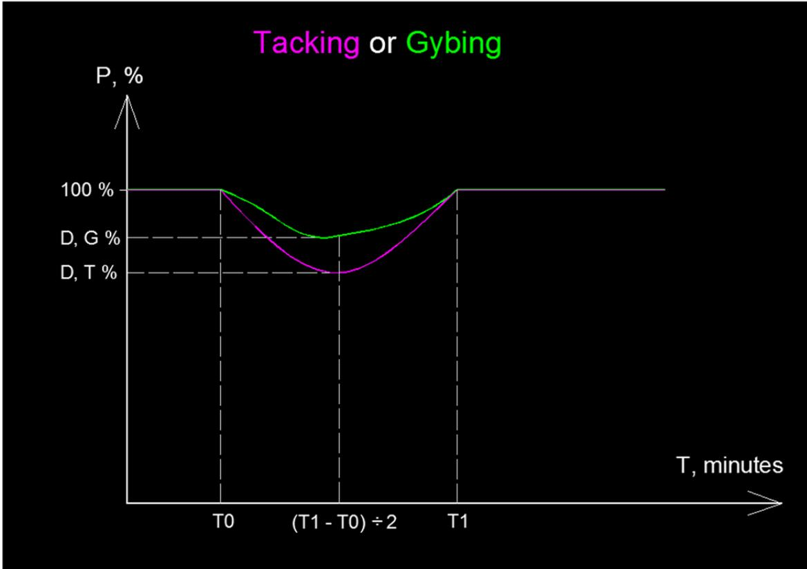
These alternate changes on BS or boat “deceleration” (decreasing of BS) / “acceleration” (increasing of BS) process during the made maneuver result from, first, the simple process of changing direction in relation to the initial path, and second, from changing the boat engine inputs via the TWA/TWS couple.
